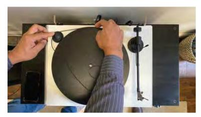
3. Rotate the platter with your right index finger while holding the belt in place until the rotation is complete and the belt is in position.
