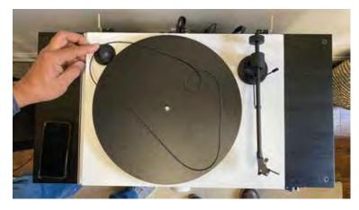
2. Locate the belt along the edge of the platter with your right index finger. Make sure the belt will not get snagged on the center post in the next step.
