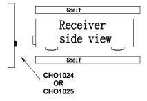
IR emitter is attached to rack door, round shape side facing the IR window
