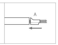
Cut excess wire at the end of the load bar (A).
