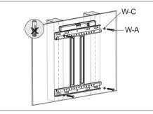
4. Attach the mount arm to the back plate
