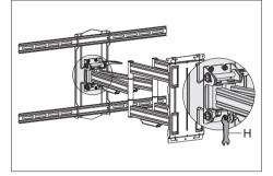
2. Level, mark & drill 1/2" holes for each anchor/screw
