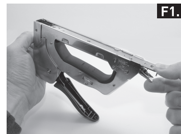
F1. Squeeze track release and pull out Exprimir soltar la pista y extraer
